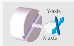
Groove finish cutting using the Y-axis
